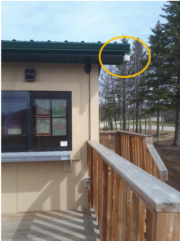
Figure 15: PurpleAir® sensor installed
